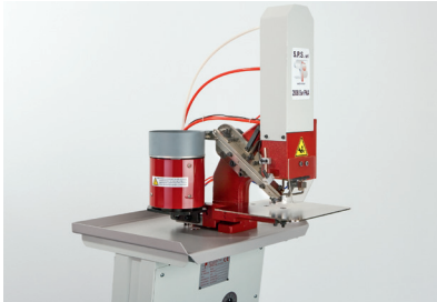
Some Swarovski products can be applied using a semi- or fully- automatic attaching machine (e.g. Rose Pins). In this process, the feed on the machine must be adjusted to the product being processed.
